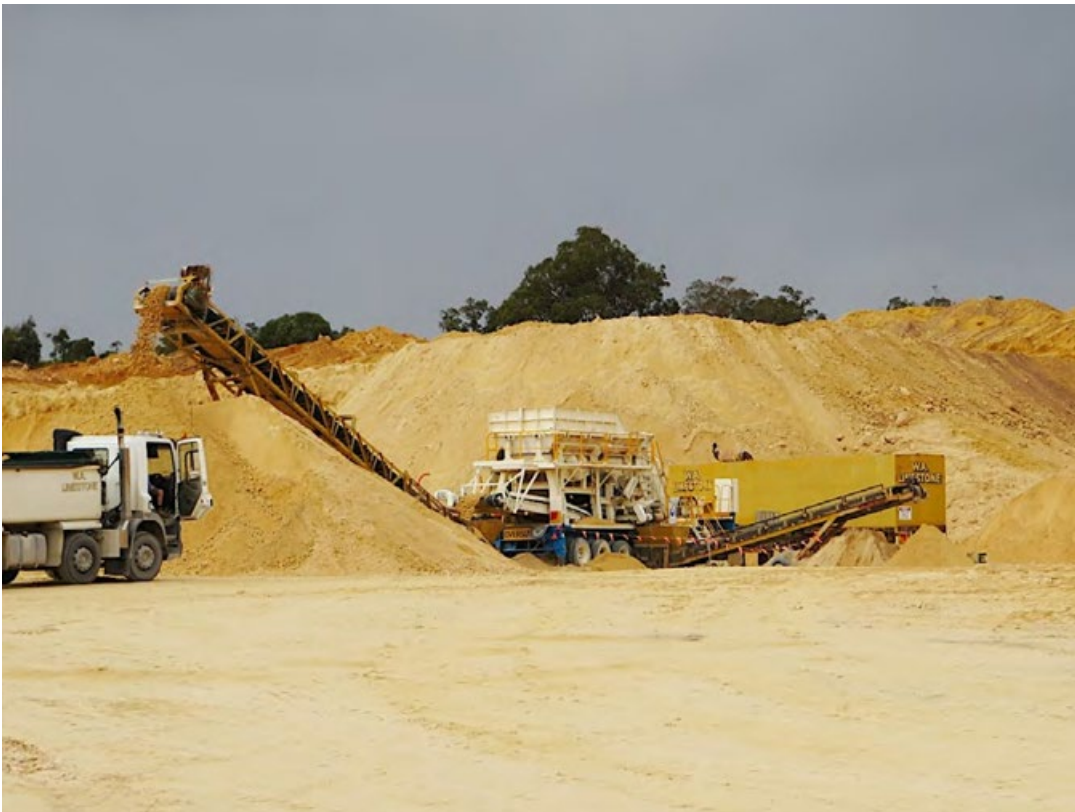
Figure 2: Crushing, screening and stockpiling operations
